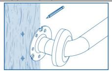
Place grab rail on wall in line with studs and mark location of screw holes.
