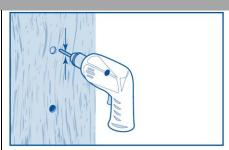
After marking, drill small hole to confirm location of stud.
